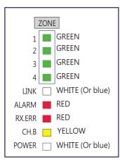
CH.B : Channel selection POWER Indicator: Normal power input when showing
