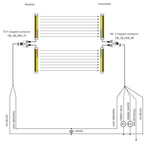
Aux. output is NPN output, max. current 20 mA.
