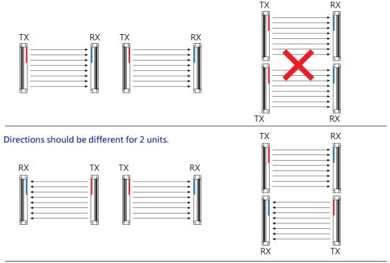
If directions are the same, place an opaque board in the middle of two units.
